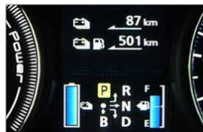
Image showing the EV travel distance on the PHEV dash board instruments.
