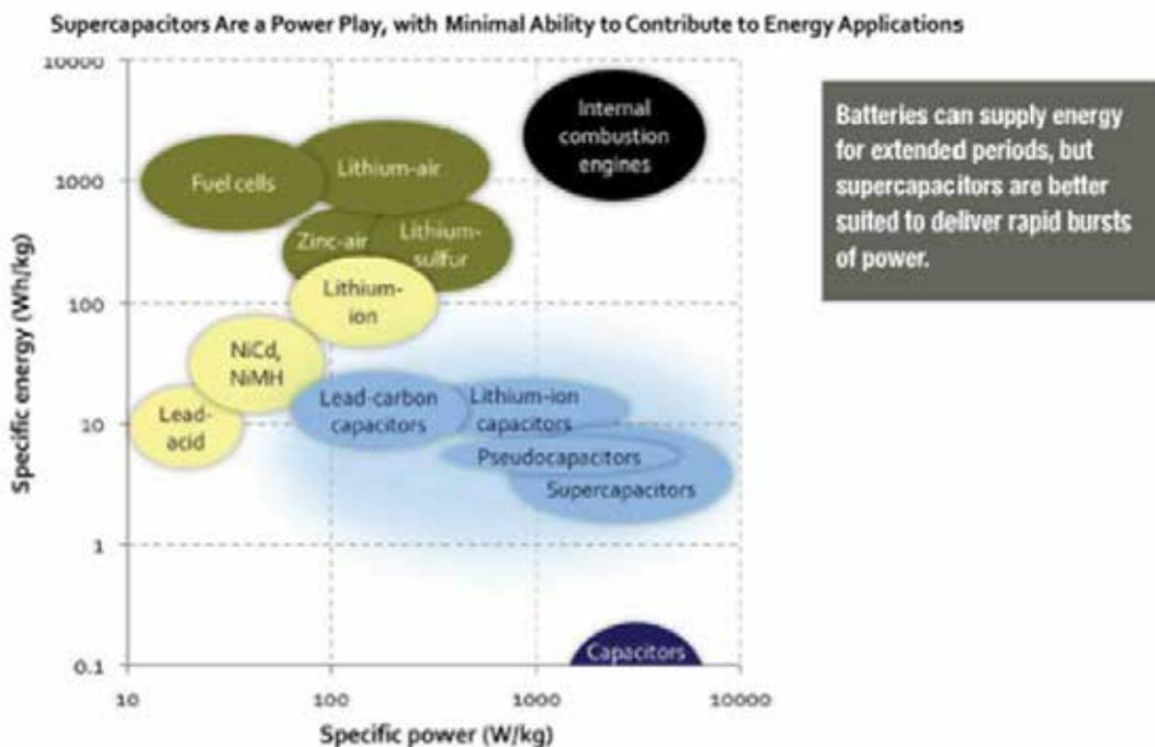
**Table T** - Comparison of properties of secondary batteries and electrochemical capacitors
