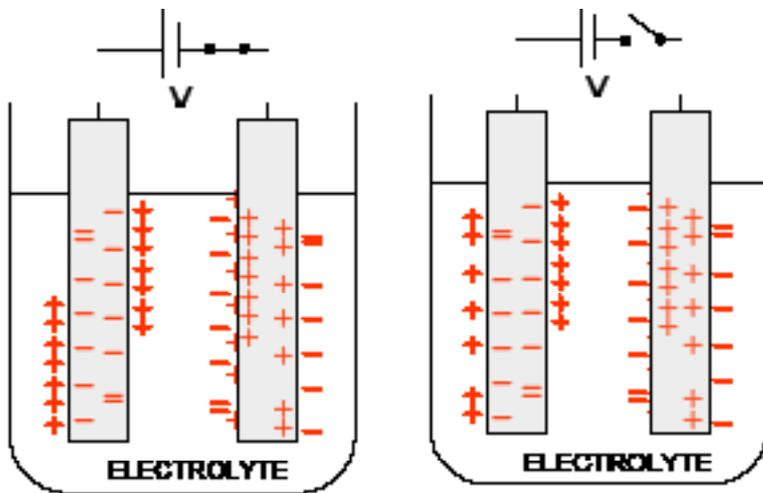
**Figure 1:** Electric double layer capacitor constructed by inserting two electrodes in a beaker and applying a voltage. The voltage persists after the switch is opened (right), creating two series-connected capacitors. Charges in the electric double layer are separated by only about 1nm.
