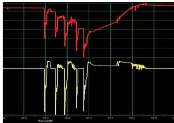
**SuperCapacitor Discharge – Cranking an ICE:**
